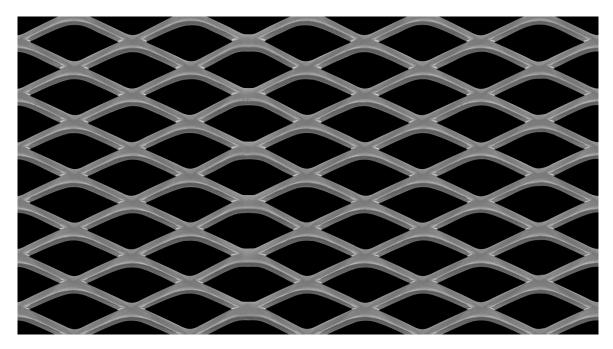
LW Pitch:30.48mmStrand Width:3.00mmSW Pitch:14.00mmThickness:2.00mmWeight:2.31 kg / m2Open Area:57%
